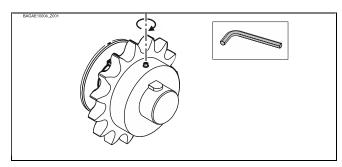
Tighten the fastening screw of the sprocket.
