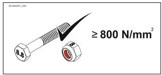
Use connection elements with a minimum strength of 800 N/mm2 (8.8).
