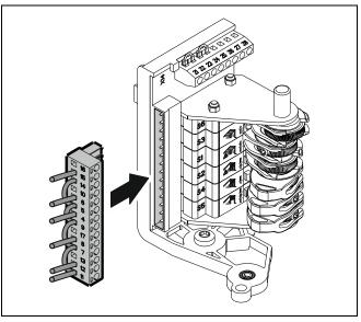
• Connect the limit switch plug.
