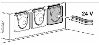
The universal brake must be supplied and controlled externally with a voltage of 24 V DC.
