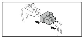
Connect the power supply to terminals X13-11 and X13-12.
