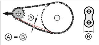
Tension the chain. The slack side (A) must not exceed the height of a chain link (®).
