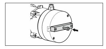
Turn the screw into the centre hole of the guide rail as far as it will go. The guide rail lifts out of the groove.
