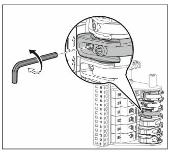
Turn the screw for fine adjustment on cam S1 until the door stops without risk even when passing the final limit positions.
