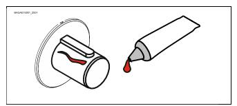
Grease the output shaft and key thoroughly. Use suitable assembly grease.
