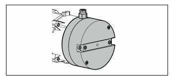
In the case of a fire, the universal brake opens and the door closes. For the duration of the assembly of the door, the universal brake can be switched to the assembly operating mode.
