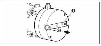
Remove the screw from the hole on the side next to the guide rail (1).
